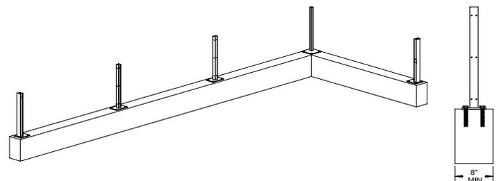
7. If the concrete is not level, washers may be placed over anchor bolts and before shoes are bolted down to serve as leveling devices.
